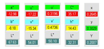
These numerical value displays show the color coordinates and brightness values that are calculated from the tristimulus values **X**, **Y**, **Z**.
