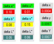
These numeric value displays show the deviations of the individual color coordinates and of the brightness value of the current surface from the "color hit" (C-No:) in the **TEACH TABLE**.
