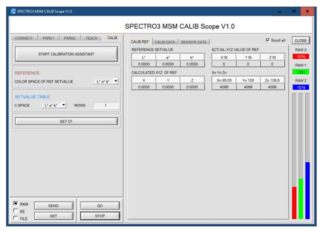
With **START CALIBRATION ASSISTANT** you can start an assistant that guides you through the calibration. The following three conditions must be met:
