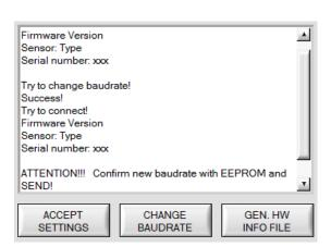
When the new baudrate information has been successfully sent, the sensor operates with the new baudrate. A window will pop up, prompting you to select **EEPROM** and then to press **SEND**. After a hardware reset the new baudrate only will be used when **EEPROM** and **SEND** have been pressed.
